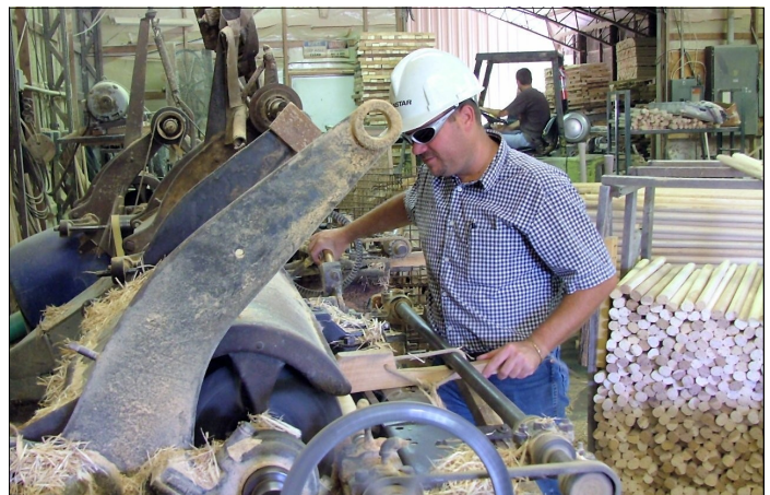
Chris House operating the sledge lathe
